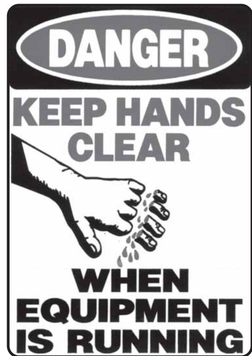
THIS LABEL LOCATED NEAR THE BELT GUARD!
